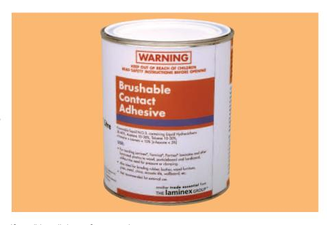
If possible, roll the surfaces together through a pinch roller or press with a rubber hand roller from the centre out to eliminate air pockets. Full bond strength will be achieved in about two days from bonding; however, about 90% of the bond strength will be obtained within 24 hours of bonding.
